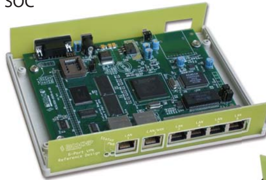
6-Port VPN Reference Design ( with Ethernet Switch)
